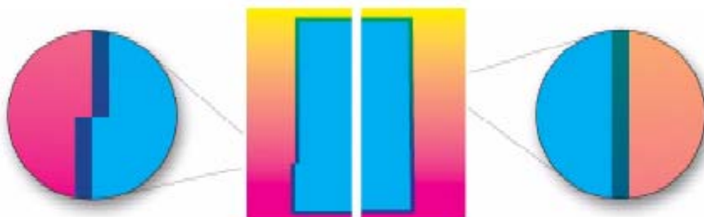
(b) Sliding trap. Notice how the trap does not have an abrupt shift in direction.
